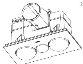
The Ducted Instant Heat 3-in-1 are ceiling mounted heat lamp appliances combining the functions of heater, extraction fan and luminaire.
